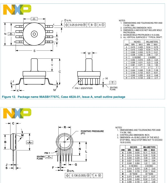
Figure 13. Package name 98ASB42793B, Case 867-08, Issue N, unibody package
