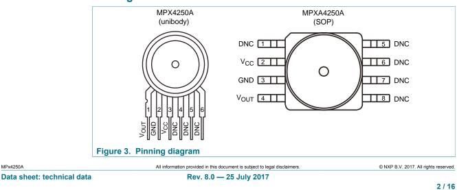
20 to 250 kPa, Manifold absolute pressure sensor, on-chip signal conditioned, temperature compensated and calibrated
